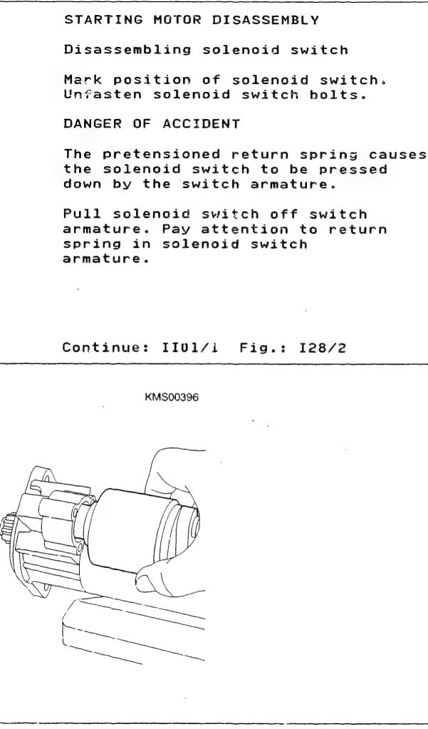
Disassembling solenoid switch
